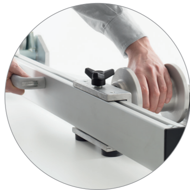
Adjust the movable counter rollers according to the drum's diameter.
